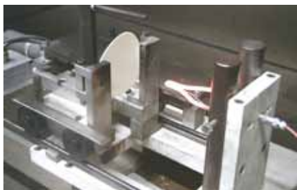
Figure 3: Glow wire test setup
